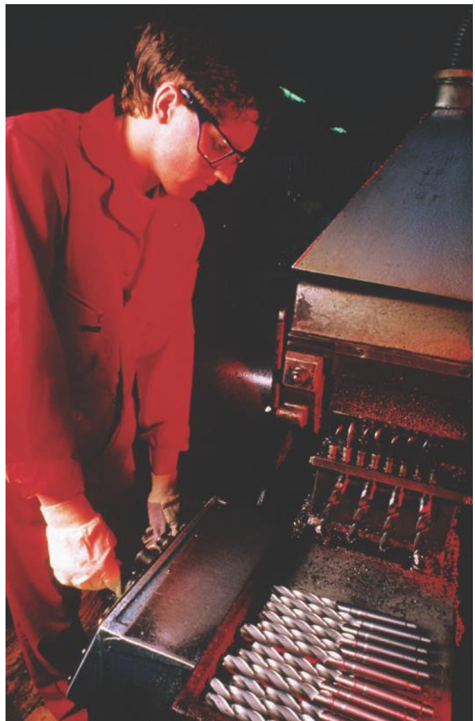
Flute milling of taper shank drills
