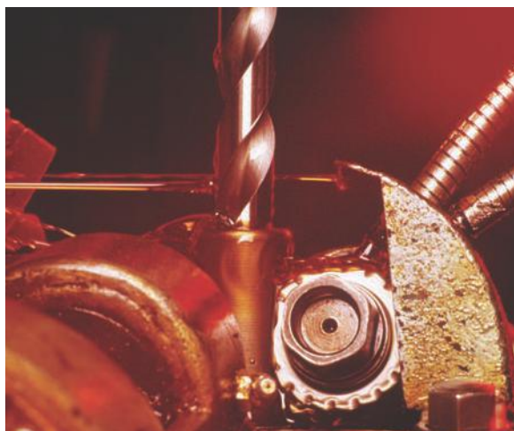
Flute milling of large diameter twist drills
