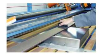
The new VSM non-woven web on cloth backing can be used with lever operated contact rollers or lever operated and hand held contact pads. It is recommended for flat and lightly profiled parts made of stainless steel and standard steels as well as non-ferrous metals. It has been specially developed for grinding on long belt machines – with all the advantages of VSM non-woven material.
