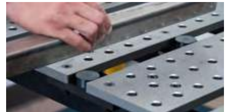
Mount the Channel Block and insert the Rest Button to create a continuous work surface over the table slot.
