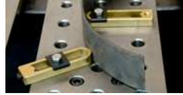
Use the round end to hold against curved or odd shaped stock.
