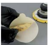
of the Rhynogrip discs from the machine's backing pad for reuse.
